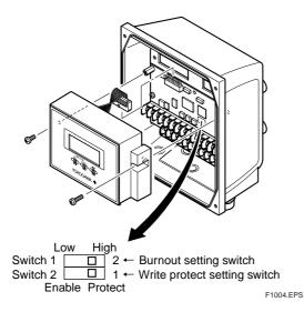
Figure 10.1.4 Switch Configuration
